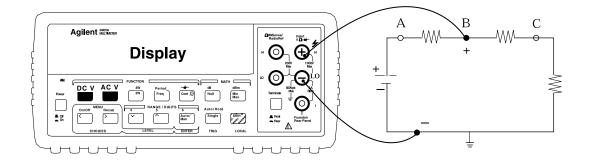
The example below shows how to measure VBC (VBC is positive):
