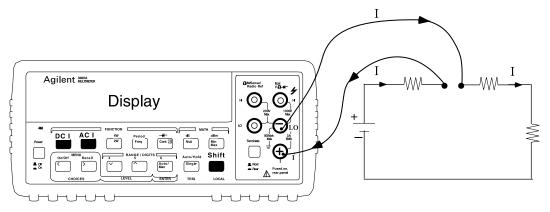
The input resistance of the ammeter is 0.1  $\Omega$  for the 1A and 3A ranges, and 5  $\Omega$  for the 10 mA and 100 mA ranges. This means that it will not load the circuit and result in a large measurement even for most resistance values (100 k $\Omega$  to 2  $\Omega$ ).
