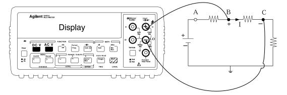
The input resistance of the voltmeter is 10 M $\Omega$ . This means that it will not load the circuit and result in a large measurement error if the resistances are 300 k $\Omega$  or smaller (see lab report assignment).
